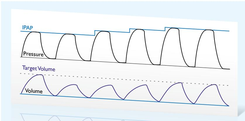
AVAPS combines the comfort and leak compensation of pressure mode and the safety and efficiency of guaranteed average tidal volume.
